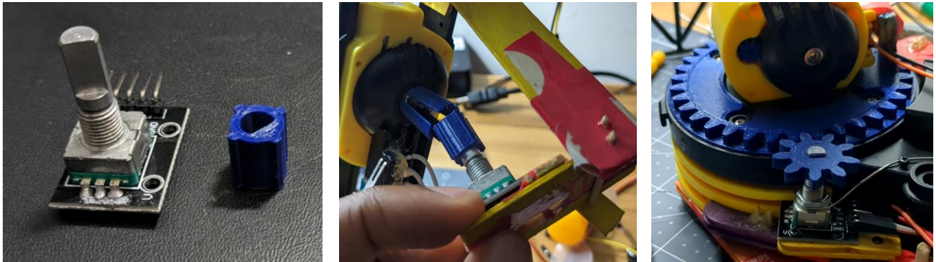
Figure 3: Interfacing the encoders with the Robotic Arm Edge
